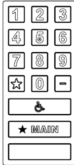
Figure 9: Functional sketches of passenger interfaces inside the cab when the car stops for its first demand from an office floor. KONE's renderings for the project are essentially the same in function, so those are not shown; credits for elements such as keypad buttons used in our sketches go to Dewhurst.
