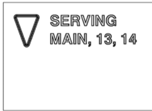
DISPLAY IN BOTH CAB FRONT RETURNS (ABOVE CAR OPERATING PANEL AREA)
